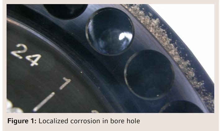
Figure 1: Localized corrosion in bore hole
